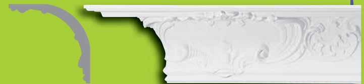
MD 1320 • 7" Projection • 6 7/8" Height • 6'6" Length • Use on centre of wall • 15" of smooth moulding on each end
